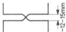
Fig. 5: Bending of the interconnection cables
